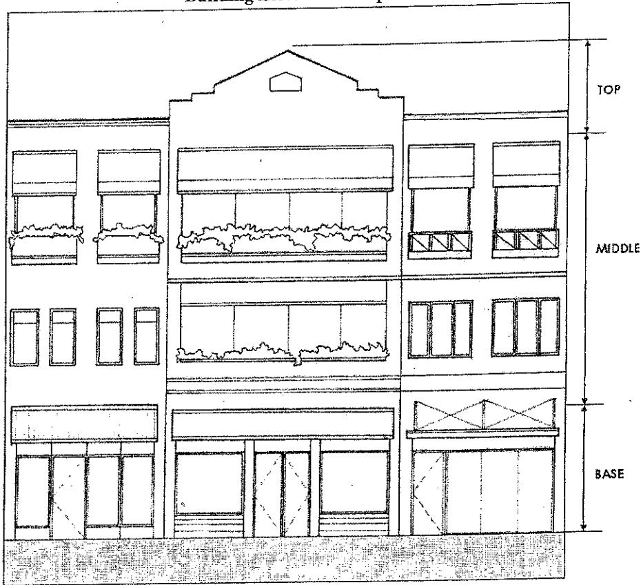
Figure 4-6 Building Elevation Composition
