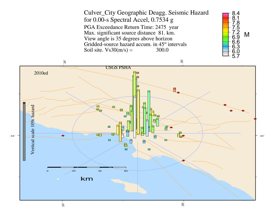
\*\*\* Deaggregation of Seismic Hazard at One Period of Spectral Accel. \*\*\*
