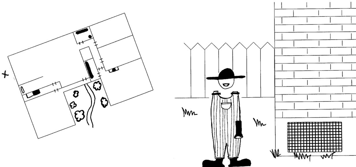
If your home is built on a raised foundation, the drain pipes are generally accessible from the crawl space. Before you enter the crawl space, draw a floor plan of your house, noting the location of the shower, bath, washing machine, and bathroom sinks. Under the house, identify which drain lines serve which fixtures and decide which ones you would like
