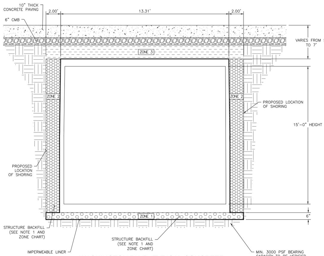
**WASHINGTON BLVD: TYPICAL CONCRETE SUBSURFACE STORAGE TANK SECTION**
