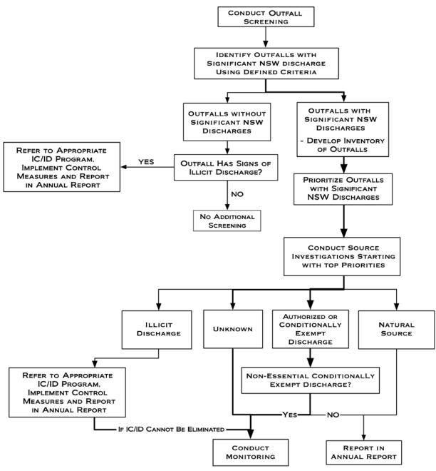
Figure 4. NSW Outfall Program Flow Diagram
